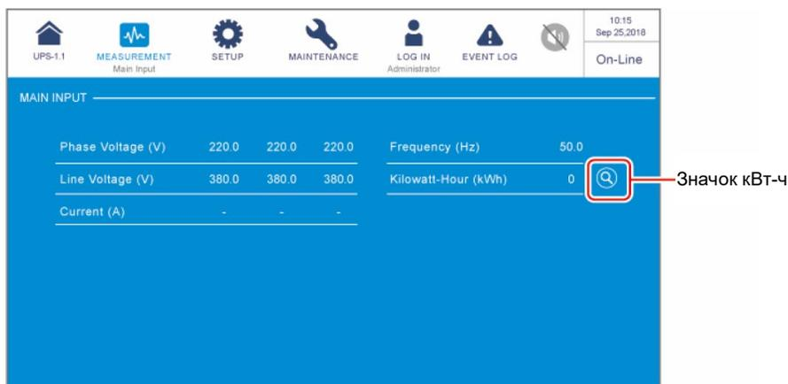
The screenshot shows the 'MAIN INPUT' page of a monitoring interface. At the top, there is a navigation bar with icons for 'UPS-1.1', 'MEASUREMENT Main Input', 'SETUP', 'MAINTENANCE', 'LOG IN Administrator', 'EVENT LOG', and a status indicator 'On-Line'. Below the navigation bar is a table of electrical parameters:
